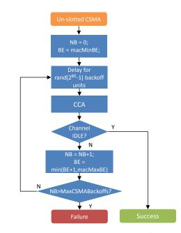
Fig. 3: Un-slotted IEEE 802.15.4 CSMA/CA algorithm
