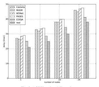
Fig. 8: AODV packet delivery latency
